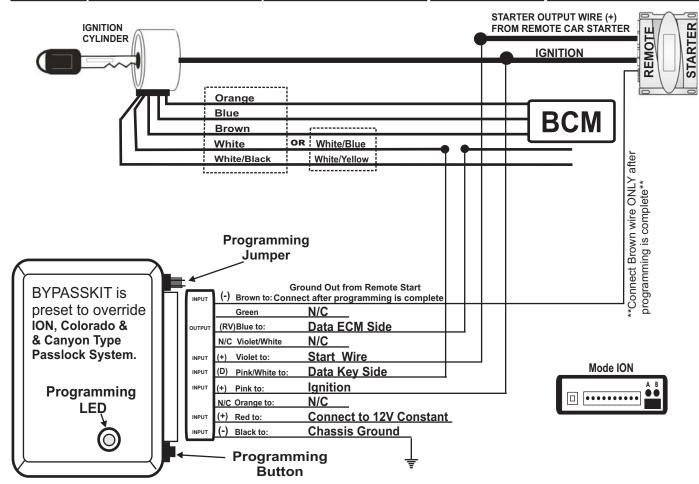
**INSTALLATION NOTES:** \*Saturn ION, GMC Canyon & Chevy Colorado etc do not have starter wires. \*\*Be sure to verify the PASSLOCK type selection on this self learning kit matches your vehicle prior to installation, otherwise the kit will not function.
